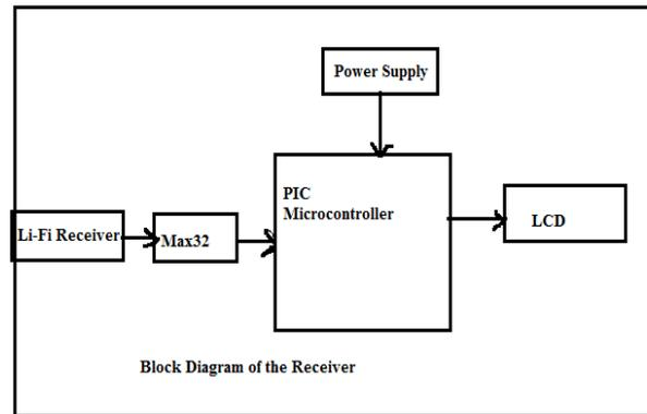
Fig.2. Block diagram of the receiver
